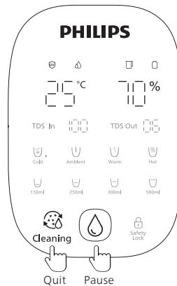
(5) When "100%" flashes, the cleaning process is completed.
